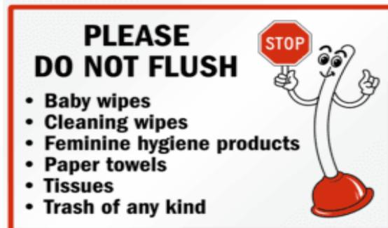
**GREASE:** Along with not flushing the above listed items, we also strongly recommend not rinsing grease down your sinks as it can/will coagulate and solidify around the impeller on your grinder pump resulting in, at a minimum, diminished pumping capacity or even worse, total failure.
